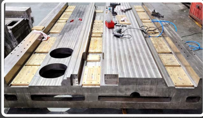
TÜM EKSENLERDE HİDROSTATİK KIZAK SİSTEMİ COMPLETE MACHINE WITH HYDROSTATIC GUIDES
