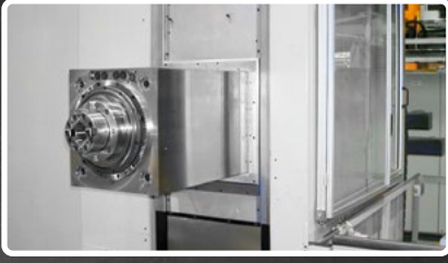
Z - RAM KESİTİ 460 x 460 mm CROSS-SECTION OF RAM
